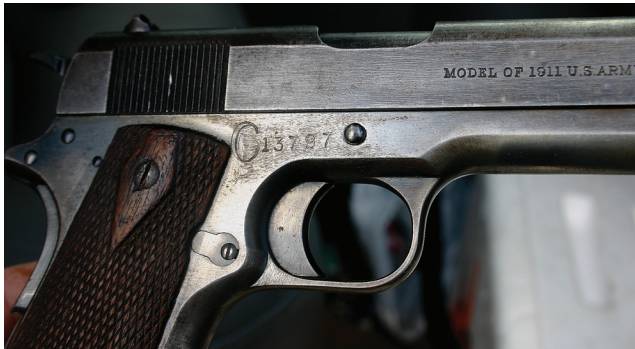
Figure 5.3 This 1913 vintage Colt 1911 has had its original serial number ground from the frame, and it has been renumbered. It is apparent that this was historical and likely done at the factory or at a government arsenal. The United States Property marking has also been obliterated from the frame by grinding and then stamping a series of X's across that part of the frame. Students of the 1911 will note the crude stamping as well as the die being inconsistent with that used by Colt. (Image from author's collection.)
